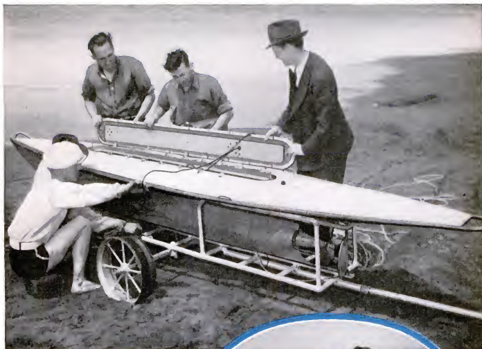
The "electric fish" on its launching dolly. Right, controlling its movements from the switch box on the shore, by means of the cable
